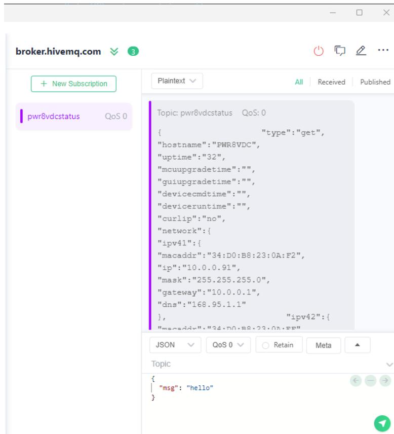
**Please note:** Not all APIs are available for MQTT control. At the moment we are limited to one line of feedback, therefore control options are mainly intended for outlet settings. Controls which apply network changes, resets, or reboots are not available for MQTT control as this could break communication and compromise functionality. The APIs can be found at the back of manual.
