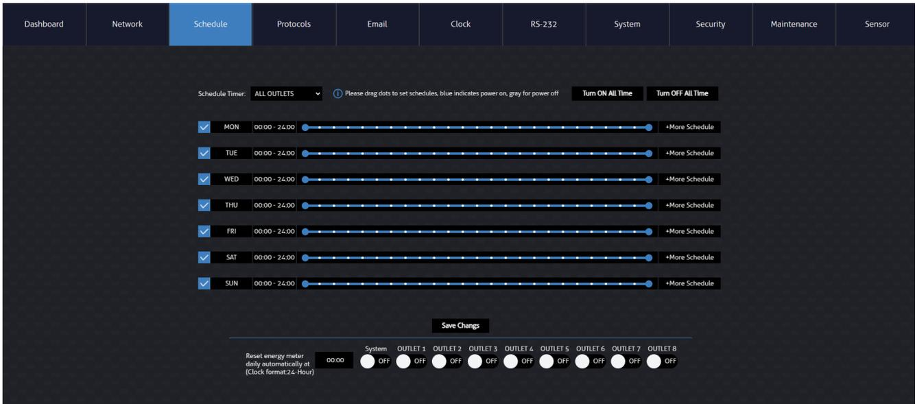
To adjust the logic for any given day, move the blue dots along the timeline to create a highlighted selection: this is when the device will power on. In order to add additional logic (i.e multiple on and off periods), press the + More Schedule button. You can now add additional logic by repeating the steps above. Press the - Delete Schedule button to remove unwanted logic.
