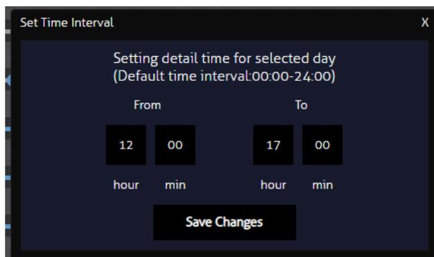
Additionally, the energy meter on the dashboard can be automatically reset at a specified time for a unique selection of outputs. Input a desired time at the bottom of the page and select the output meters to be reset daily at that time.
