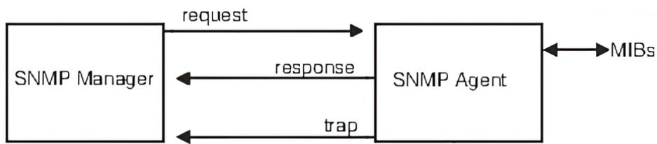
The PWR8VDC acts as an SNMP agent and can be configured to communicate with an SNMP manager of your choice.
