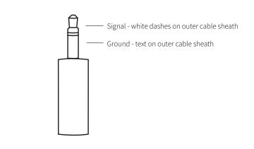
IR Receiver - IRR (1.45m cable length - not including connector or receiver bud)
