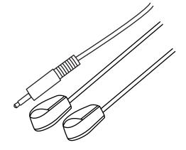
If having to splice together multiple IR cables to provide extra emitter diodes, or extending/shortening cables, this is done so at the users own risk. The 5V IR line provided by Blustream equipment will only have a set amount of current to drive the IR emission to the diodes. "Splitting" this signal multiple times, or extending over a longer cable will decrease the strength of the signal.
