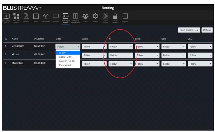
By default, each IR route is set to "Follow" the HDMI video data from TX to RX. Using the drop down selection in the IR column of the example above, a fixed route can be made from the transmitters IR Input to the IR output of a receiver by selecting the relevant transmitter for each zone.
