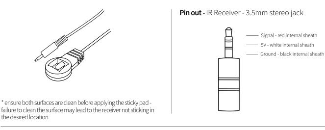
IR Link Cable - IR-CAB (1.95m cable - not including connectors)
