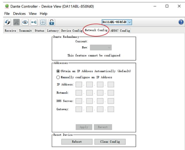
It is also possible to change the settings of the DA11ABL-WP-US under the “Device Info” screen in the Dante Controller software. To do so, select the “Device Config” menu.
